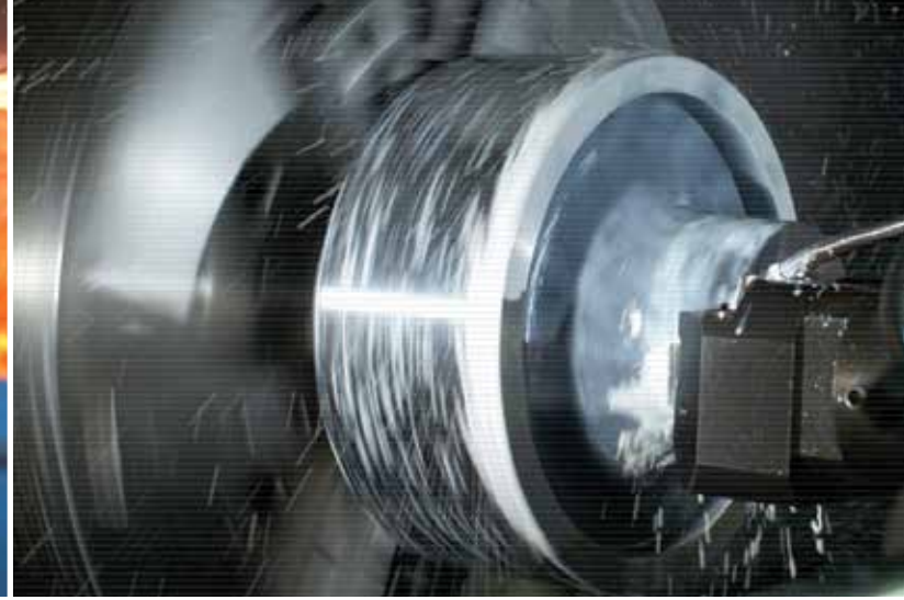
Brake wheel during turn complete operation.
