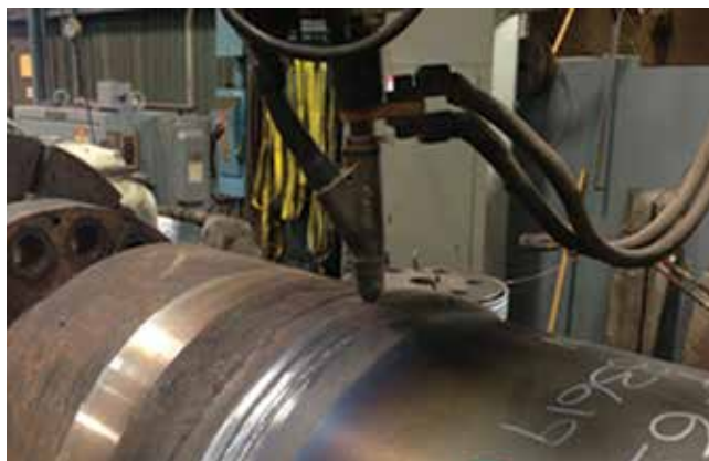
Coupling adapter and spindle weldment assembly, during the submerged arc welding (SAW) process. In many cases reconditioned gear coupling assemblies require that replacement components are joined to modified components. All welding processes at Xtek are tightly controlled and utilize superior welding wires and flux combinations to produce the desired metallurgical properties.
