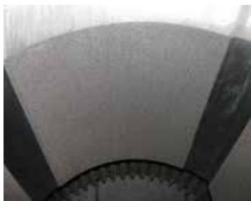
The as-machined surface of a TSP Roll End Casing following the Electro Discharge-Machining (EDM) process.
