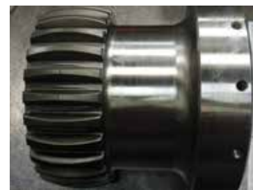
Splined coupling adapter and hub gear at final inspection.
