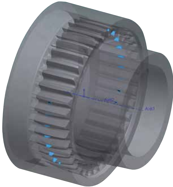
Model and FEA showing wear pattern and stress concentration points in a coupling ring gear and hub gear at a 3° operating angle.
