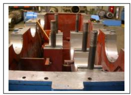
The gearbox was disassembled, inspected, and evaluated:
