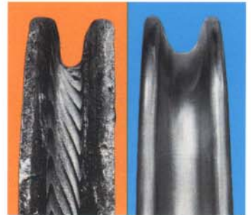
Competitor's wheel (left) showing severe corrugation after a few month's service. An Xtek sheave wheel (right) still on the job after 3 years in the same application.
