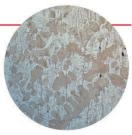
Optimal Hardness Working Layer 67-72 HSC (50-54 HRC)
