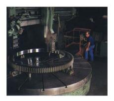
**Shaping** generates gear teeth with either a pinion or rack shaped cutter, removing stock from the face of the gear blank in a reciprocating action, while the blank slowly indexes. Spur, helical, herringbone and internal gear teeth are generated on machine tools manufactured by Fellows, Sykes and Maag, among others.
