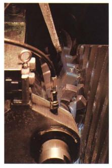
**Form Grinding** is another method of improving geometric accuracy of a previously machined and heat treated gear. Form grinding uses a single grinding wheel, contoured to the shape of the desired space between teeth to reduce distortion which occurs during heat treatment. Form grinding is operationally equivalent to milling, and can be performed on both spur and helical external gears.
