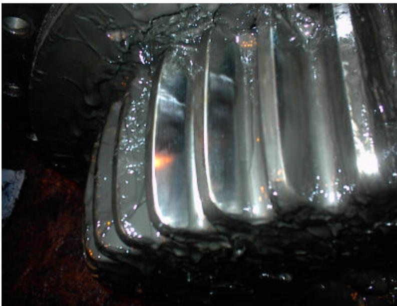
Properly lubricated gearing after 1 year tour-of-duty in a hot strip mill
