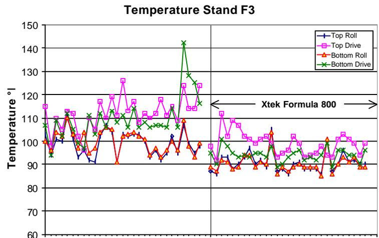
Proper lubricant and lubrication procedures greatly increase the life of a gear coupling. Using Xtek Formula 800 Coupling Compound on a regular basis will significantly improve the performance of Hot Strip Mill coupling assemblies. Xtek recommends that you:
