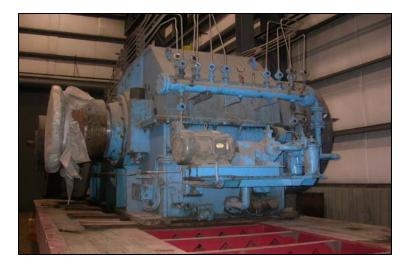
A critical component in modern thin strip steel mills is the Caster Shear Gearbox. Located at the base of the Continuous Caster, this gearbox shears a 2" thick by up to 80" wide strip of steel to the proper length for processing in the Hot Strip Mill.
