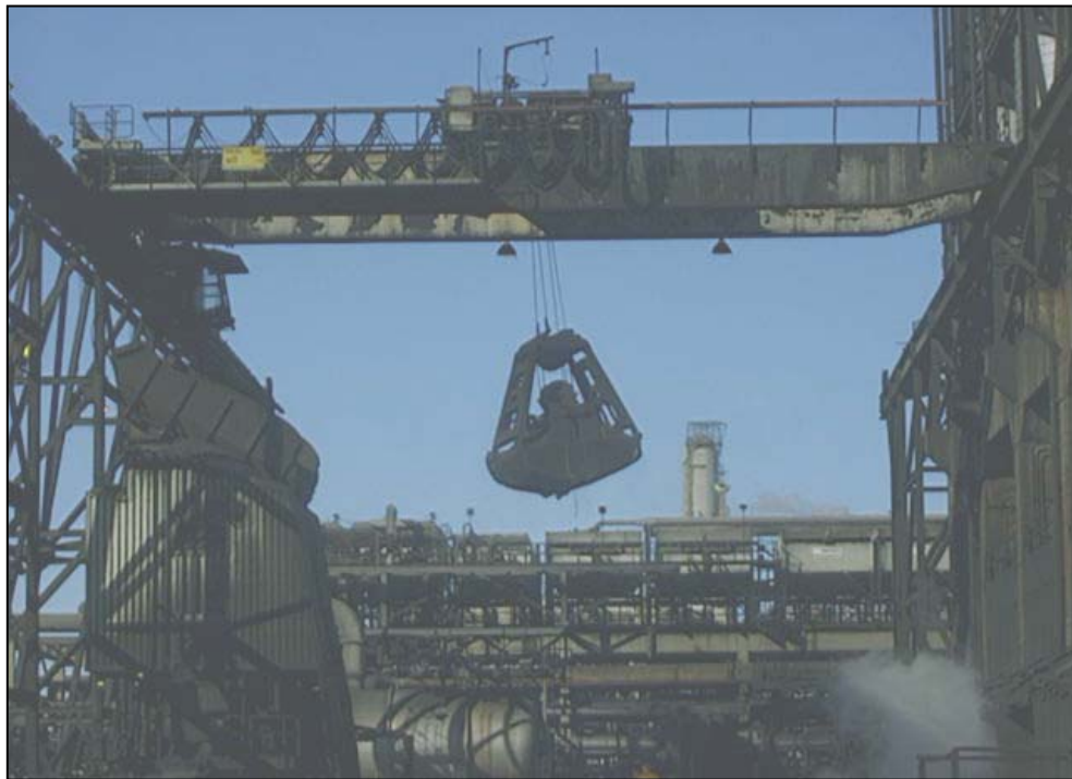
CLAMSHELL BUCKET - LOADING COKE
