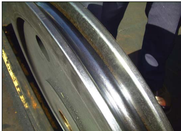
XTEK TSP CARBURIZED SHEAVES AFTER TWO YEARS OF SERVICE NO WEAR, NO CORRUGATION
