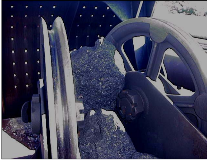
WORN FLANGE AND THROAT OF AN ORIGINAL SHEAVE WHEEL RESULTING IN FREQUENT REPLACEMENT OF ROPE AND SHEAVES
