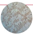
Optimal Hardness Working Layer 67-72 HSC (50-54 HRC)
