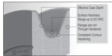
Advanced Xtek carburized and hardening processes ensure substantially longer life for our wheels plus this reduces wire rope wear resulting in much less downtime and fewer parts replacements. Our customers see real cost savings and increases in productive time.
