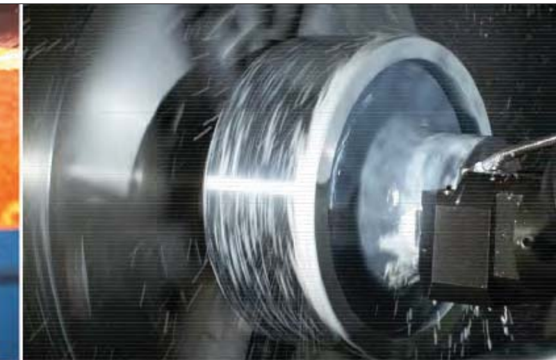
Brake wheel during turn complete operation.
