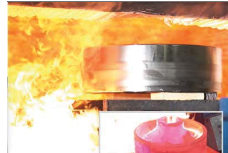
Brake wheel entering and exiting heat treating furnace.
