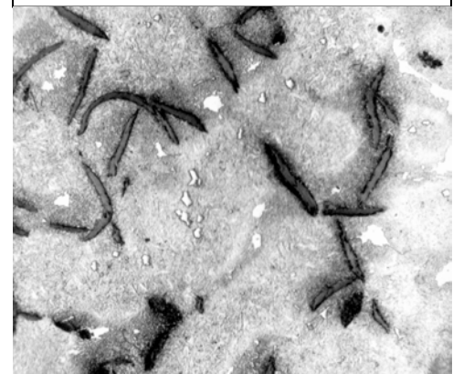
Figure 3. Representative photomicrograph of Bemcalloy C-141 microstructure, 500X (Courtesy Xtek, Inc.)
