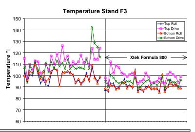
Proper lubricant and lubrication procedures greatly increase the life of a gear coupling. Using Xtek Formula 800 Coupling Compound on a regular basis will significantly improve the performance of Hot Strip Mill coupling assemblies. Xtek recommends that you:
